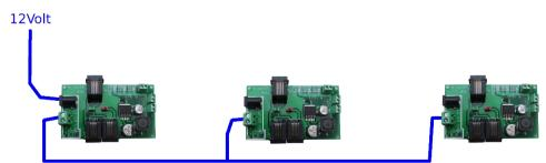
The LocoNet contacts can be used as normal LocoNet branching contacts.
