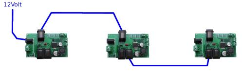
The jumper "JP3" should be connected, as it connects two wires in the LocoNet cable, thus doubling the maximum current that can be transported in the cable.
